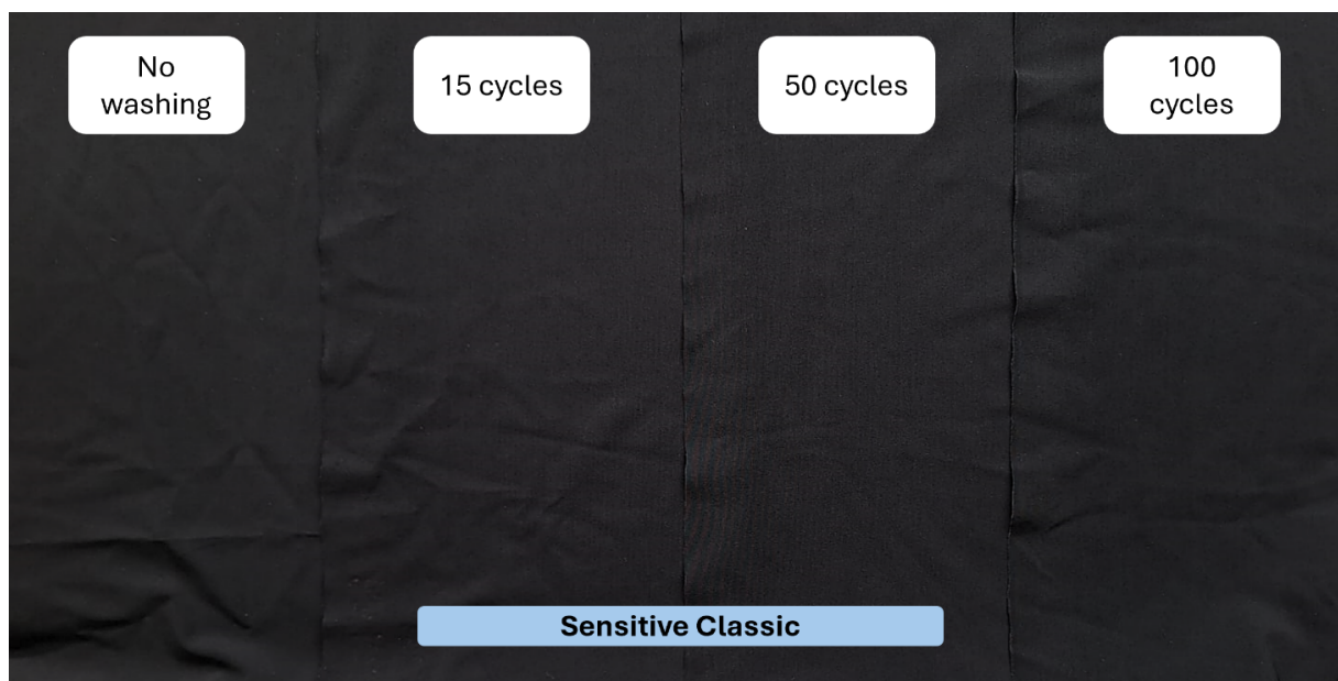
Figure 1. Appearance of Sensitive Classic fabric samples before and after 15, 50, 100 cycles of washing and drying.
